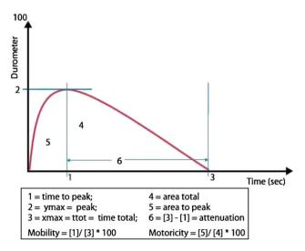
**Figure 2** Portion of a hysteresis graph used to calculate a Durometer by the SA201<sup>®</sup> durometer equipment (courtesy of Thomas Rustler, MD; Vienna, Austria).
